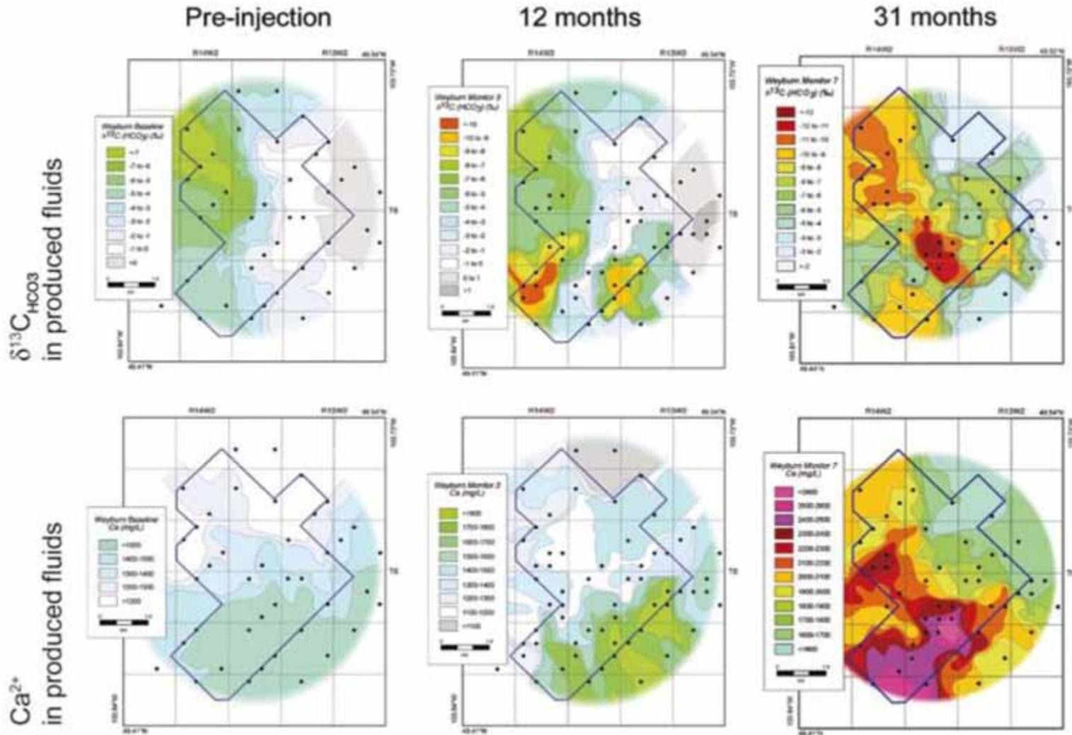
Produced water chemistry at Weyburn (Source: Perkins et al., 2005)
