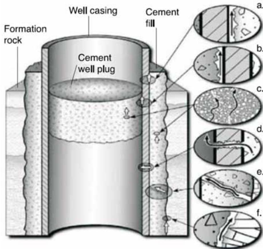
Possible leakage pathways in an abandoned well
